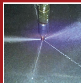
Poor spray pattern with clogged injector.
